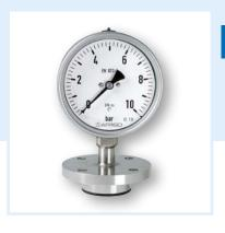
Application Flange type diaphragm seal MD 56 for sterile process separation of pressure measuring and control units in pipes or tanks. For mounting to Bourdon tube pressure gauges, pressure transducers and pressure switches. For installation in sterile processes without dead spaces. Typical application areas:
