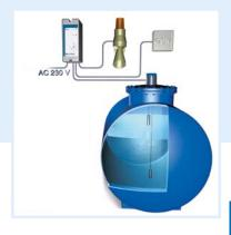
Application Suitable for use with electrically conductive liquids whose level is to be limited or controlled. The liquids such as water, emulsions or waste water must neither foam excessively nor be viscous or adhesive (bridging). CoFox® ELT 8 can be operated with one probe as a level switch or with two probes for controlling pumps, vales, etc (start/stop). Can also be used as a water alarm unit, for example in control stations or IT rooms, in conjunction with floor water probe BWS 10-1.
