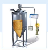
For continuous level measurement in containers, tanks or silos. Suitable for liquid, powdery, granular, electrically conductive or non-conductive media. Ideal for changing media. Also suitable for pressurised or vacuum tanks.
