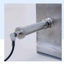
Application For non-contact level detection through metal pipe walls or metal tank walls. SonarFox® USG 22 is ideal for applications involving highly ultra-pure liquids. Retrofitting is possible even while the system is filled, the process does not have to be interrupted. Optimal for applications in the pharmaceutical and food industries.
