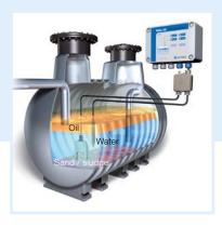
Application WGA 04 monitors oil, petrol and grease separators for accumulations of sand and sludge and generates an alarm signal when it is time to clean the separator. WGA 05 additionally monitors the thickness of the layer of separated liquid and generates an alarm signal when it is time to drain the separator.
