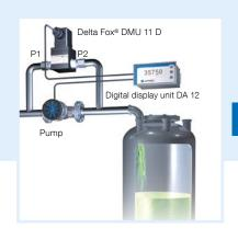
For electronic differential pressure measurement in industrial applications. For corrosive gaseous and liquid media which are not highly viscous and do not crystallise.
