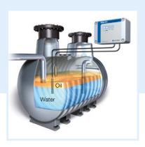
Application Oil and petrol pose a great hazard to groundwater and waste water. WGA 01 monitors the thickness of the layer of separated liquid in oil and petrol separators and generates an alarm signal when it is time to drain the separator. In addition, the maximum level in the separator can be detected. This avoids overfilling that may be caused by clogged outlets or other circumstances. The unit keeps harmful substances from reaching the sewage water system.
