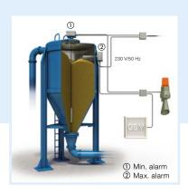
For detecting levels of powdered and finely grained bulk solids or of liquids. Especially suitable for use in silos, hoppers, tanks and containers.
