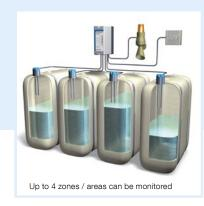
Application Suitable for use with electrically conductive liquids which do not foam excessively, are not viscous and not adhesive (bridging), e.g. water, emulsions or waste water. Ideal for generating alarms in large installations and facilities. Several zones (also large areas) can be monitored simultaneously with electrodes (probes) at various points.
