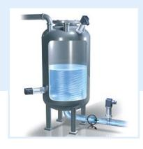
Application Suitable for detecting limit levels in liquids with a maximum dynamic viscosity of 10,000 mPa ● s and a minimum density of 0.7 kg/dm³. Specially useful in applications in which float switches cannot be used due to liquid flow, turbulence or product adherence. Ideally suitable as an overflow alarm or for dry-run protection. Due to the WHG approval, VibraFox® can be used as part of an approved overfill prevention system.
