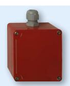
**Description** For monitoring the oxygen concentration and toxic gases. Can also be used in dusty and dirty environments. For connection to the gas alarm units GW-S 2.1/GW-S 4.1/GW-SK 6.1. Aluminium version for wall mounting housing. Connection cable (shielded) 3 x 1.5 mm<sup>2</sup> Cu+ protective conductor, signal and return conductor (max. 100 Ohm line resistance).
