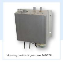
Application For dew point reduction of humid gases to help avoid condensation in the analyser. A stable gas outlet dew point avoids water vapour cross sensitivity and volumetric errors.
