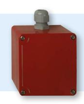
**Description** For the detection of flammable, explosive, toxic gases or oxygen. Can also be used in dusty and dirty environments. For connection to the gas alarm units GW-S, GW-S4 and GW-SK. Aluminium wall mounting design. Connection cable (shielded) 3 x 1.5 mm<sup>2</sup> Cu+ protective conductor, signal and return conductor (max. 100 Ohm line resistance).
