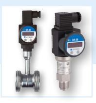
Application Cost-effective digital display unit with local indication for all transducers with 4–20 mA output and ISO 4400 (DIN 43650-A) connector. Easy and fast mounting via plug-in system. Optional EX protection (zones 0/1) and connector M 12 x 1, 5-pin.
