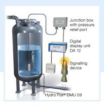
Application For electronic, continuous level measurement in extremely corrosive liquids, e.g. chemicals or waste water from landfill sites.
